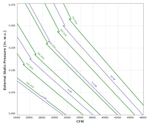
Max Sizeable RPM = 730 RPM. Curve shown extended beyond this point for reference only.
